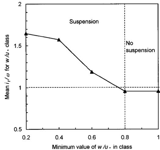
**Fig. 2.** Graph of mean value of  $i_t/\omega$  for each  $w/u_*$  class against minimum value of  $w/u_*$  for each class. Graph is based on data from 155 experiments with  $\theta > 0.6$ .
