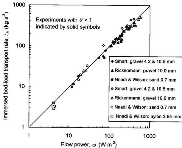
**Fig. 3.** Graph of immersed bed-load transport rate against flow power for experiments with sheet flow ( $\theta > 0.6$ ) and no suspension ( $w/u_* > 0.8$ )
