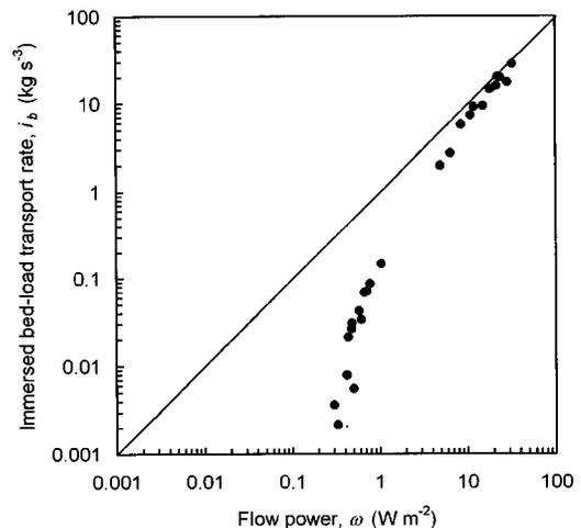
**Fig. 1.** Graph of immersed bed-load transport rate against flow power for 26 flat bed experiments by Williams (1970). Flow power was calculated using data for hydraulic radius due to bed provided by Williams (1970, Table 2).
