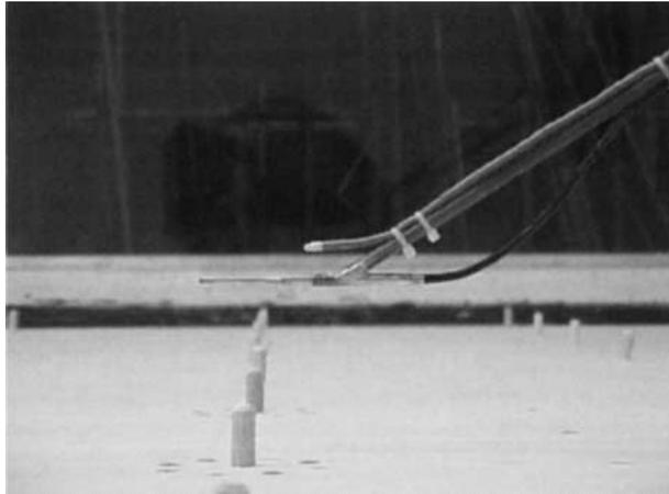
Figure 4. Photograph of the hot wire probe.
