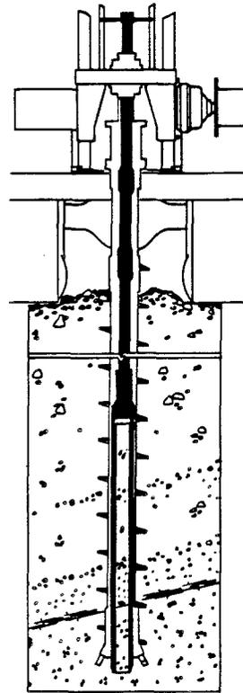
Fig. 1. A diagram of the split, hollow-tube cores mounted within a drill used in obtaining deep cores in the rooting zone of mesquite *Prosopis glandulosa*
