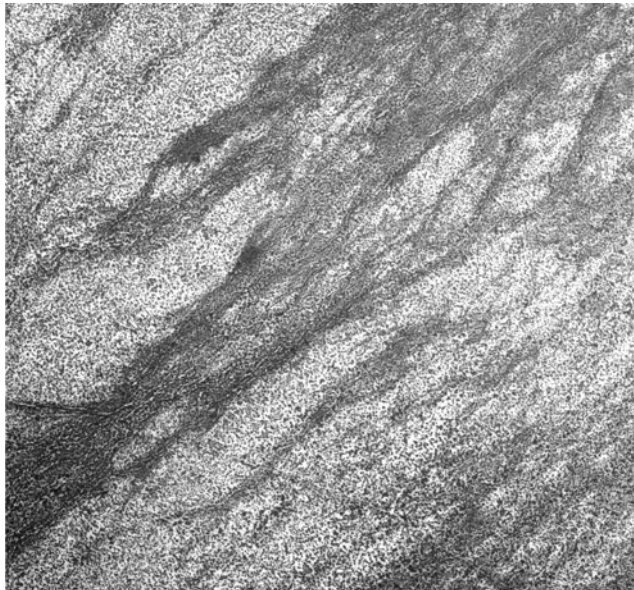
Figure 4. Aerial photograph over the Jornada Experimental Range in October 2006 showing runoff flow paths after rainfall events at 25-cm resolution. Flow paths are darker because of an increase of surface soil moisture.
