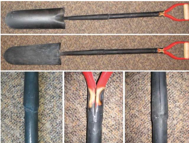
**Figure 2.** Modified shovel emphasizing new welds.
