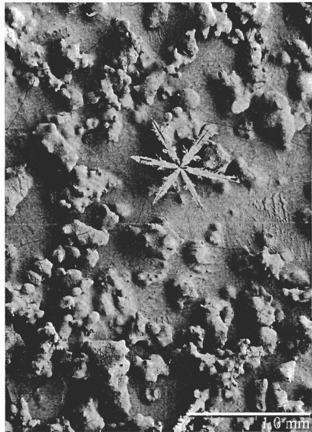
FIG. 1 Artificial snow collected in the plume of a snow gun. Artificial snow appears as small ice pellets. Natural snow, falling at the time of sampling, resulted in the fortuitous presence of the stellar dendrite along with the artificial snow. Sample collected at Sugarbush, Vermont.
