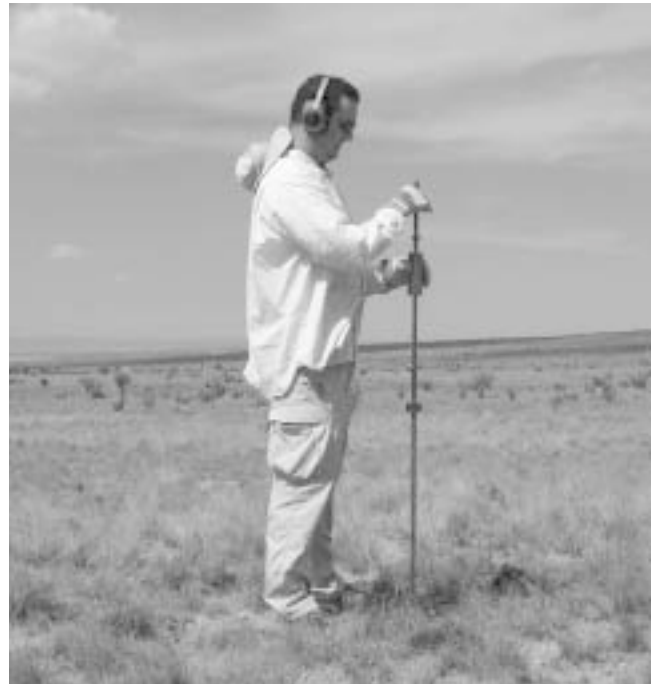
Figure 7.1. Impact penetrometer with sliding hammer elevated.
