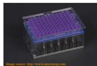
Figure 1. MicroResp™ assembly showing deep well plate on the bottom which contains whole soil samples supplemented with various carbon sources. A detection plate (made with agar, sodium bicarbonate, potassium chloride, and cresol red) is placed on top, with a porous rubber seal sandwiched between the two plates. Typical reactions are left to incubate for 6h after which the detection plate is read in a spectrophotometer.
