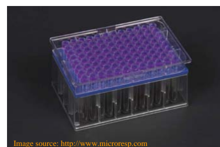
Figure 1. MicroResp™ assembly showing a deep well plate on the bottom which contains whole soil samples supplemented with various carbon sources. A detection plate (made with agar, sodium bicarbonate, potassium chloride, and cresol red) is placed on top, with a porous rubber seal sandwiched between the two plates. Typical reactions are left to incubate for 6h after which the detection plate is read in a spectrophotometer.
