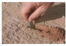
Figure 13. Excavate small trench.
