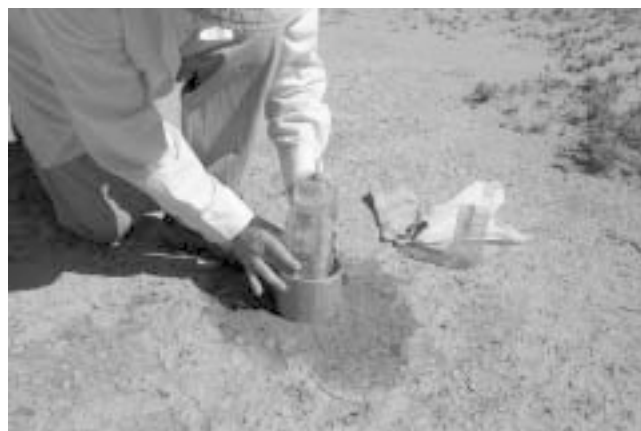
Figure 8.7. Suspend bottle inside the ring.
