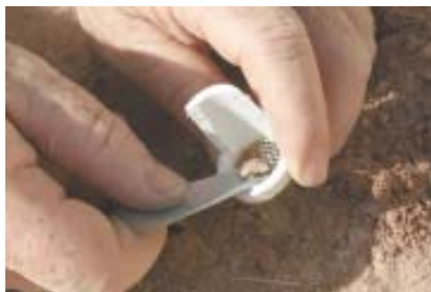
Figure 16. Place sample in sieve.
