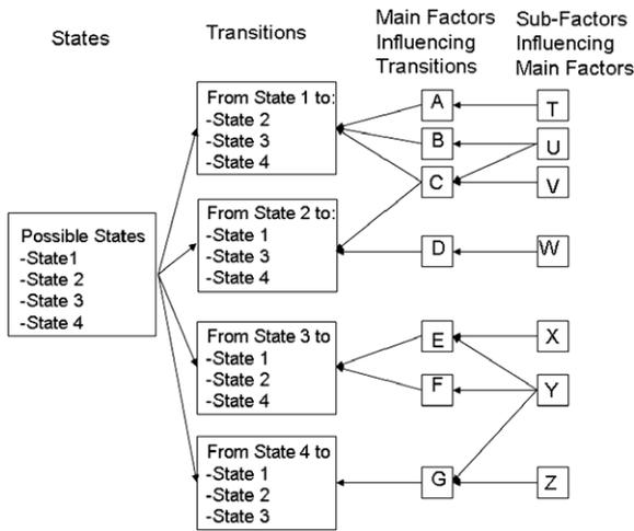
Fig. 2. Framework used to construct an directed acyclic graph from a state and transition model.
